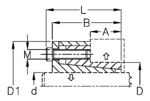
A mm = 27 B mm = 46.0 D1 mm = 57.0 d H8 mm = 20 D mm = 38 F kN torque = 34 L mm = 52.0 M mm = 6 P N/mm2 surface pressure on shaft/hub = 81 T N m torque = 330 Ts N m bolt tightening torque = 17
